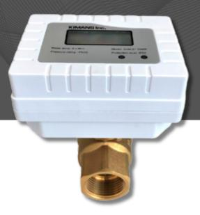
SVM-21 smart valves are battery operated open/close valves for remote disconnection by stopping flow, operating on M-Bus protocol. It comes with software for monitoring & control with error reporting functions and an IP68 protection.
