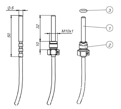
1 – temperature sensor; 2 – Temperature sensor holder; 3 – Sealing ring
