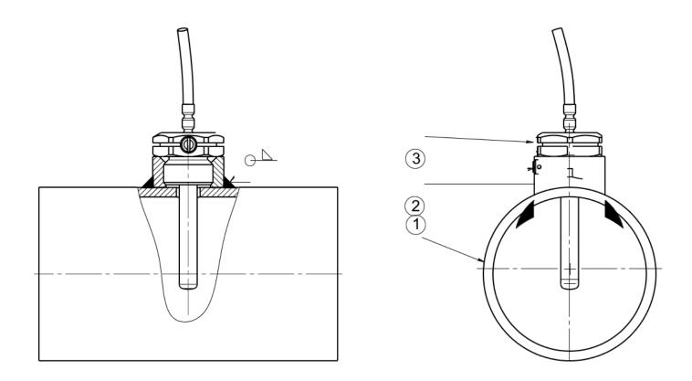
For DN greater than 50 installations of both RTD is carried out by means of a protective sleeve (pos.3), fig. below
