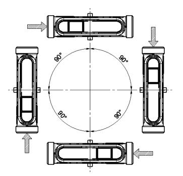
Flow metering section may be installed vertically, horizontally or at any arbitrary angle.
