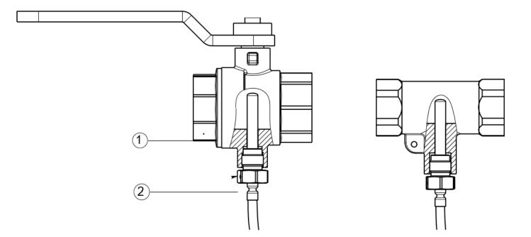
RTD can also be installed in a tee. To do this, use a special adapter (pos.3), which is directly screwed into the RTD holder (pos.2).
